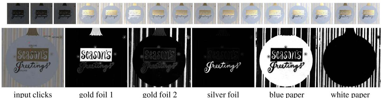
Fig. 2. KNN matting on material matting using the *sg* dataset. Original images at the top; the bottom shows sparse user input (five clicks, one per layer) and the five layers automatically extracted. Our result distinguishes the two different gold foil layers despite their subtle difference in materials (where they were combined in [11]).
